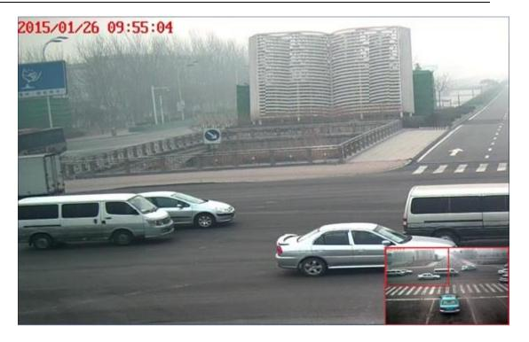
2.Use the mouse to choose magnified area, that is, to enlarge the red areas 3.Mouse wheel can zoom in and out red box area, move or choose a new red box area, can switch to the need enlarge the area.
