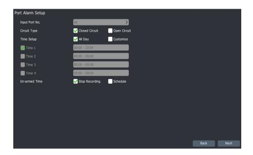
2)Under the "Port Alarm Setup], users can set alarm circuit type, time period and un-armed time operation. Click [Next] to "Port alarm recording parameters" interface.
