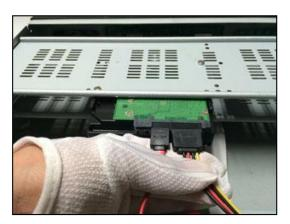
3. Connect the power cable of HDD to the power connector of the NVR.
