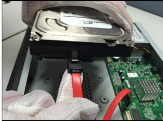
3. Connect the power cable of HDD to the power connector of the NVR.
